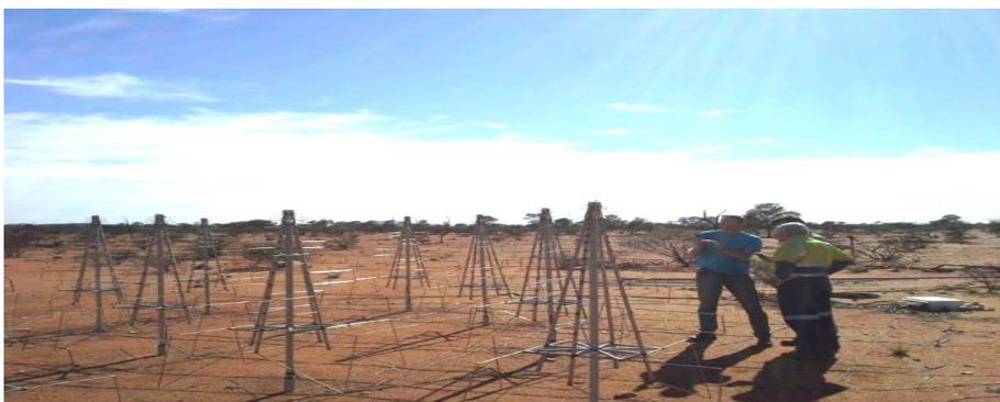
Figure 1: SKA\_Low antennas installed at the MRO for trial purposes.
